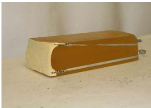
Figure 5: Ordnance gelatin used as penetration surrogate.
