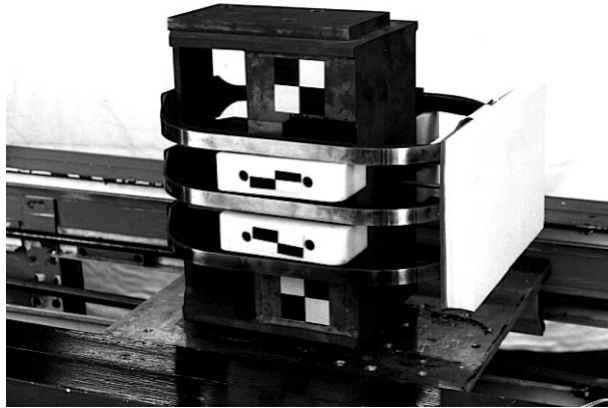
Figure 4: 3-Rib Ballistic Impact Dummy (3RBID) modified based on corridors developed by Bir et al. [9].
